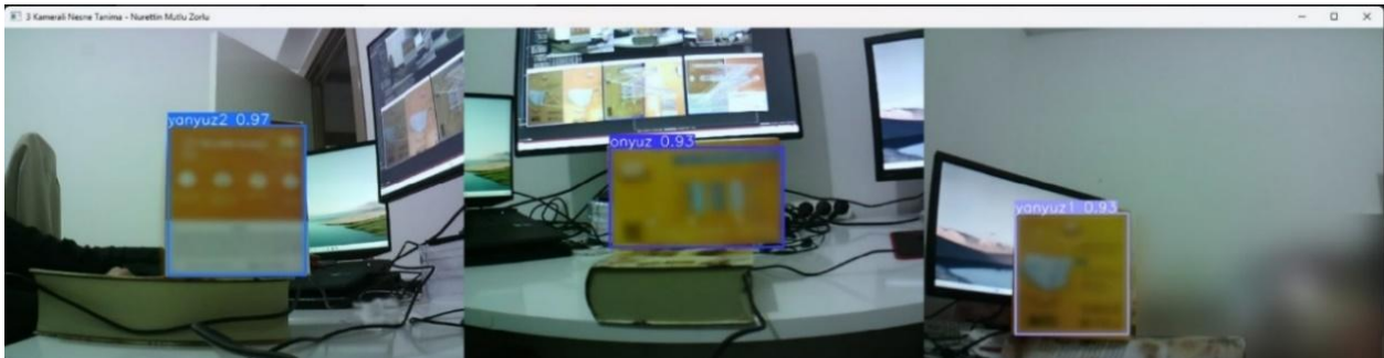
Figure 5. Object recognition from different angles with three different cameras
